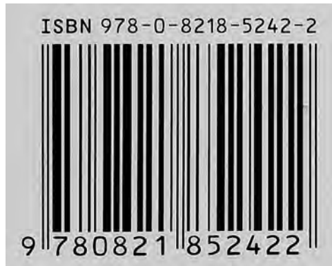
Figure 4.2. An example of a UPC-A code (below the barcode) and an ISBN-13 code (above the barcode).
